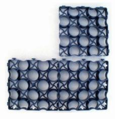
Plate 3: EASYGrid after 10 loading cycles, loaded unfilled Loading area demarked red.
